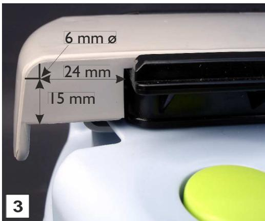
If there is not a hole in the slide handle on the ventilating knob side of the cartridge, this must be provided subsequently. Follow the dimensions according to the photo.
