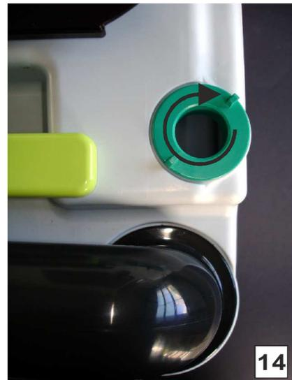
Insert SOG hose connection into the bayonet and turn right until you feel the hose connection click into place. If this appears difficult, ease in O-ring with silicone spray or some soap.
