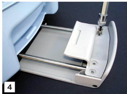
Unlock slide handle and pull on, locate cartridge in reverse position and unscrew the four Torx screws with Torx insert TX 10. Remove slide handle.
